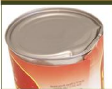
Severe dent in seam
