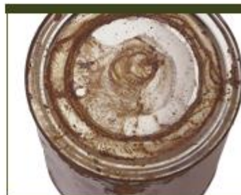
Rust that cannot be wiped off
