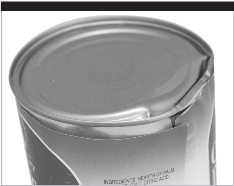
Severe dent in seam
