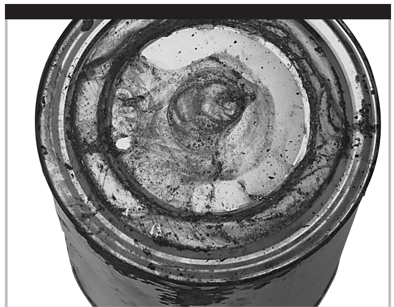
Rust that cannot be wiped off
